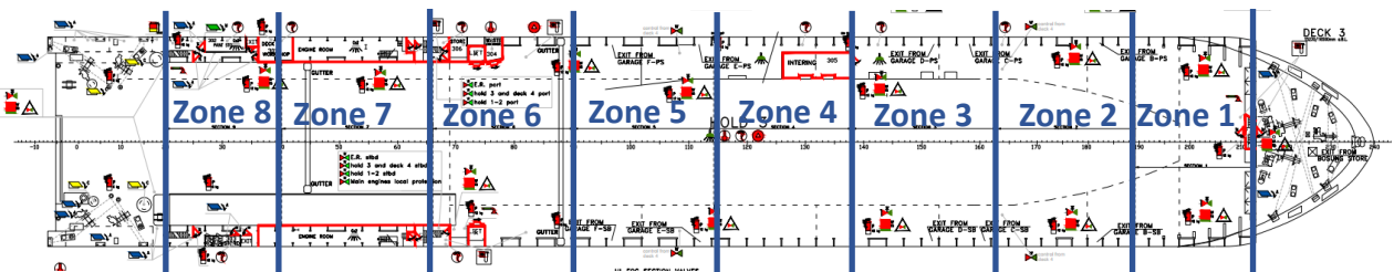
Figure 4. Abstract of Fire Fighting Equipment Plan. Blue lines indicate the operating zones of the Drencher System
